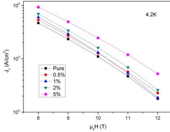
**Fig. 1.** Magnetic field dependent transport critical current density of pure and doped tapes at 4.2K. The applied field is parallel to the tape surface in the measurement.
