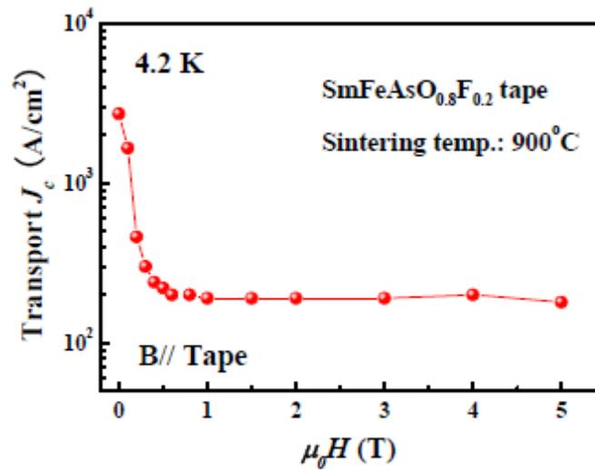
**Fig. 2.** Transport critical current density  $J_c$  at 4.2 K as a function of field for  $\text{SmFeAsO}_{0.8}\text{F}_{0.2}$  tapes heat-treated at 900°C.
