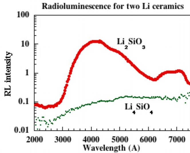
Fig. 2: IMR results for radioluminescence characterization of Li containing ceramics using proton irradiation.
