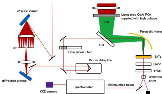
Fig. 2 Scheme of THz generation and detection.
