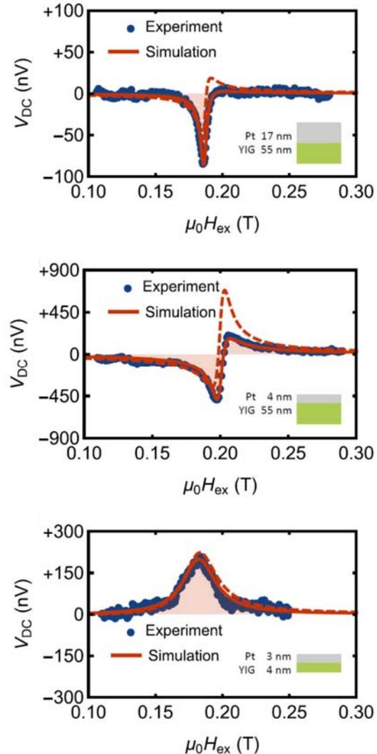
**Fig. 3:** Measured (dots) and simulated (lines) of the dc voltage generated under and ac applied current for three different YIG|Pt samples with thicknesses indicated in the insets [5]. The dashed lines correspond to zero phase shift between the Oersted magnetic fields and the applied current.
