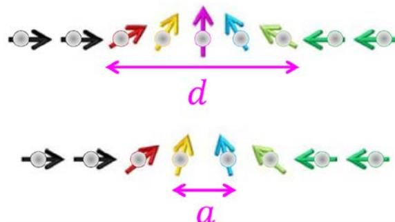
**Fig. 2:** Two head-to-head magnetic domain wall configurations with different energies illustrating the concept of atomic pinning for narrow domain walls when the domain wall width  $d$  becomes of the order of the lattice constant  $a$  [2]
