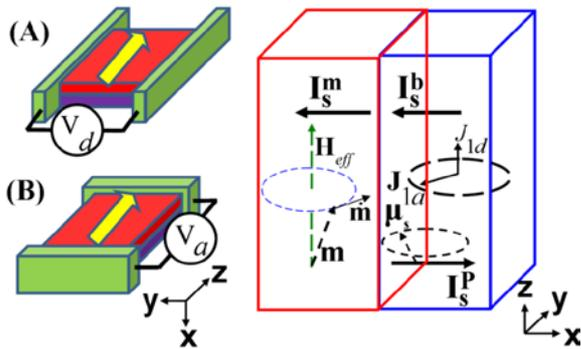
**Fig. 3:** Schematic spin battery operated by FMR for the measurement configurations (A) and (B). The AC(DC) voltage drops  $V_a$  ( $V_d$ ) along the  $z$ ( $y$ ) direction. In the right panel the magnetization  $\mathbf{m}$  (time derivative precesses around the effective field  $H_{eff}$  in the left layer, generating DC/ AC spin currents and a spin accumulation in the normal metal (right side) [3].
