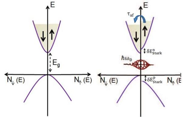
**Fig. 4:** Illustration of the changes in the majority and minority population due to the Stark shift in the presence of non-resonant and intense circularly polarized laser field that acts as an effective magnetic field to create a spin accumulation or exert torques on a magnetization [4].
