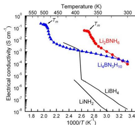
Fig. 2 Electrical conductivities of  $\text{Li}_2\text{BNH}_6$  and  $\text{Li}_4\text{BN}_3\text{H}_{10}$ . The melting temperatures are indicated as  $T_m$ . For reference, the data of the host hydrides  $\text{LiBH}_4$  and  $\text{LiNH}_2$  are also shown.
