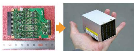
Fig. 2 photograph of evaluation system for light outputs, energy resolution: Si-Photo Multiplier.
