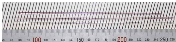
Fig.1 Photograph of fiber scintillator.
